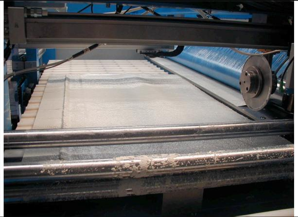
A circular knife makes a cross-cut : a dedicated piece is cut from the SMC compound (its length L depends on the desired weight of your product).
