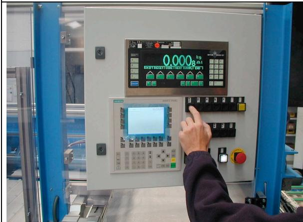
A balance precisely measures the actual weight (Ist-Wert). The machine will automatically take this weight into account, and correct the length L (if required), in order to achieve a weight (Ist-Wert) that is as close as possible from the theoretical weight (Soll-Wert). By this way, the machine automatically corrects for variation in the density of the product.
