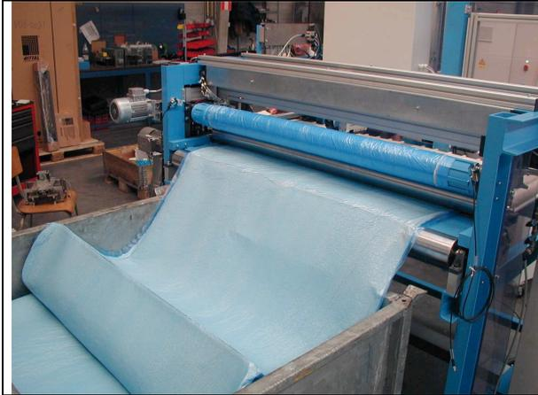
The SMC product is supplied in a container, with protective foil (in this case : width 1250mm – 400meter per container). The protective foil is removed from the compound.
