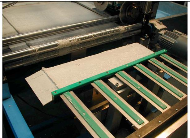
A second knife cuts the cross-cut part into individual pieces, and stacks these pieces at the output of the machine. The weight of the stack exactly matches the desired weight. A robot can take the parts from the cutting machine, and place them in the mold, under the press.
