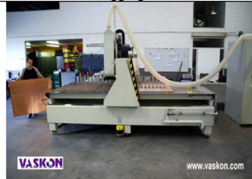
Machine equipped for pendulum operation
